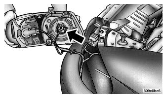
3. Disconnect the electrical connector and replace the 7 bulb.
