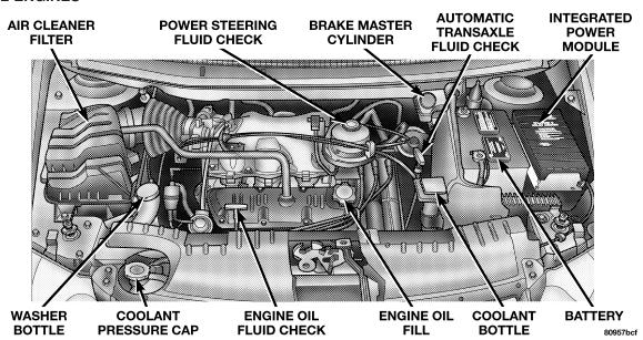
Engine Compartment 3.3L/3.8L Engines
