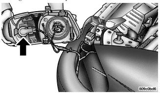
3. Replace bulb, reinstall socket and then reinstall the headlight module.
