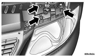
2. Turn the bulb socket retaining ring or the bulb assembly counterclockwise.
