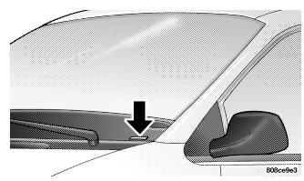
**Vehicle Identification Number NOTE:** It is illegal to remove the VIN plate.
