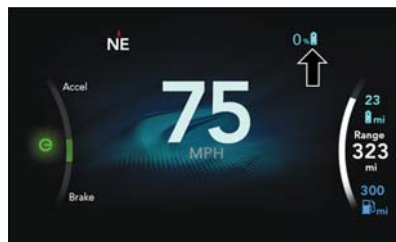
High Voltage Battery Gauge
