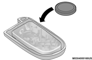
Key Fob Battery Replacement
