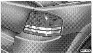
1. Open the trunk and gently pull back the trunk liner behind the taillamp.
