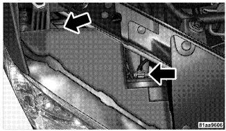
3. Rotate bulb and connector ½ turn and pull outward 4. Pull the bulb out of the socket and replace the bulb. from assembly.
