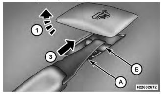
1— Cover 3— Attaching Strap A— Tether Strap Hook B— Tether Anchor
