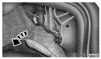
2. Remove the two plastic wing nuts from the taillamp housing.
