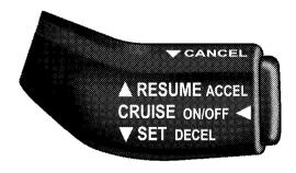
**NOTE:** In order to ensure proper operation, the Electronic Speed Control System has been designed to shut down if multiple Speed Control functions are operated at the same time. If this occurs, the Electronic Speed Control System can be reactivated by pushing the Electronic Speed Control ON/OFF button and resetting the desired vehicle set speed.
