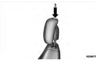
3 — Final Downward Movement To Engage Locking Mechanism
