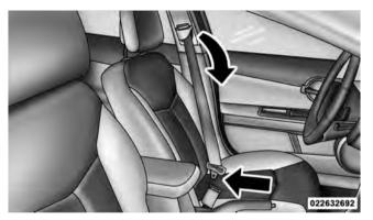
Inserting Latch Plate into Buckle
