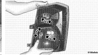
NOTE: It is not necessary to completely remove the tail lamp unit. Once loosened from the quarter panel, there should be enough room to service any of the bulbs.
