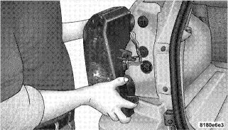
4. Twist and remove socket from the lamp.
