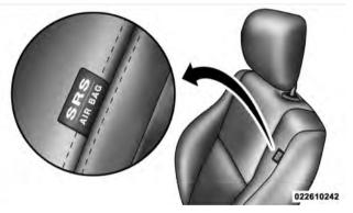
**Supplemental Seat-Mounted Side Airbag Label** When the airbag deploys, it opens the seam between the front and side of the seat's trim cover. Each airbag
