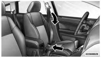
Inserting Latch Plate into Buckle
