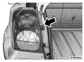
3. Disconnect the electrical connector from the bulb. 2. Grasp the tail lamp and pull firmly to disengage the lamp from the aperture panel.
