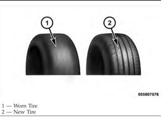
These indicators are molded into the bottom of the tread grooves. They will appear as bands when the tread depth becomes 1/16 in (2 mm). When the tread is worn to the tread wear indicators, the tire should be replaced.
