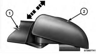
**NOTE:** The rear wiper arm cannot be raised fully upward unless the pivot cap is raised first.
