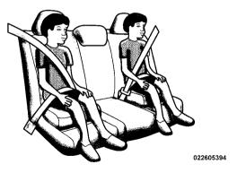
8. To remove the slack from the lap belt, pull upward on the shoulder portion of the seat belt.
