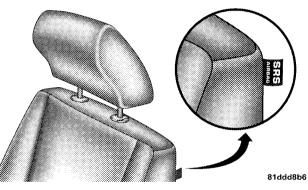
Seat Mounted Side Airbag Label When the airbag deploys, it opens the seam between the front and side of the seat's trim cover. Each airbag
