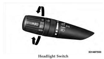
NOTE: The engine must be running before the headlights will turn on in the automatic mode.
