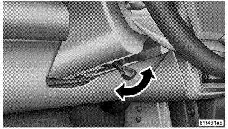
Tilt/Telescoping Steering Control Handle
