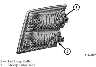
5. Remove the bulb from the connector socket and install the replacement bulb.
