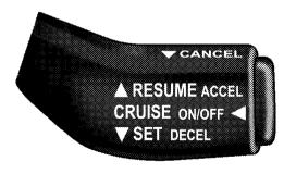
**NOTE:** In order to ensure proper operation, the Electronic Speed Control System has been designed to shut down if multiple Speed Control functions are operated simultaneously. If this occurs, the Electronic Speed Control System can be reactivated by pushing the Electronic Speed Control ON/OFF button and resetting the desired vehicle set speed.
