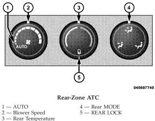
The Rear-Zone ATC for the rear passengers is in the overhead console above the second row passenger seats.
