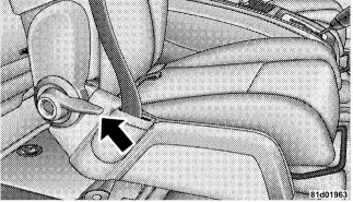
**Fold-Flat Seat** Pull upward on the lever to fold or unfold the seat.
