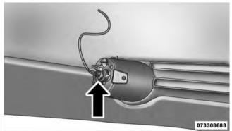
3. Remove the bulb from the connector socket and install the replacement bulb.
