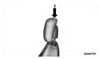
3 — Final Downward Movement To Engage Locking Mechanism
