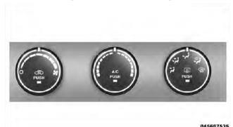
The Manual Temperature Controls consist of a series of outer rotary dials and inner push knobs.
