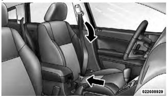
**Inserting Latch Plate Into Buckle**
