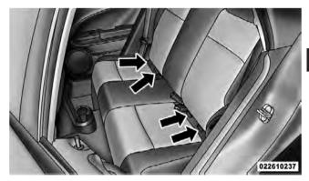
Rear Seat LATCH Anchorages Installing The LATCH – Compatible Child Restraint System
