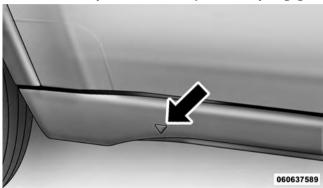
Lift Point Symbol On Sill Molding
