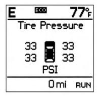
Should a low tire condition occur on any of the four active road tire(s), you should stop as soon as possible, and inflate the low tire(s) that is "flashing" on the graphic display to the vehicle's recommended cold tire pressure displayed in the "Inflate to XXX" message. The system will automatically update, the graphic display of the
