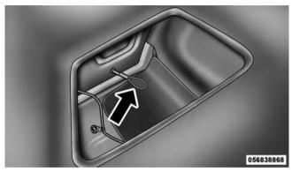
Release Cable Loose Fuel Filler Cap Message
