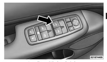
Auto Down Window Switches Auto Up Feature With Anti-Pinch Protection — **Driver And Front Passenger Door Only**
