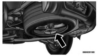
Road Wheel Installed In Spare Location
