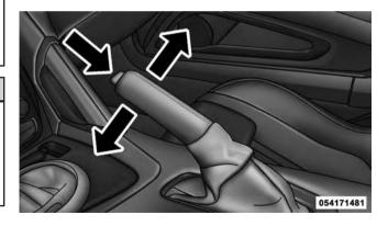
The parking brake should always be applied when the driver is not in the vehicle.
