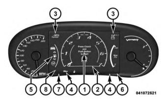
The EVIC displays are located in the center portion of the cluster and consists of the following sections:
