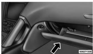
Opened Glove Box Storage Compartment NOTE: The glovebox storage compartment will lock with the door locks.
