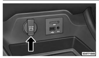
**NOTE:** Do not exceed the maximum power of 160 Watts (13 Amps) at 12 Volts. If the 160 Watt (13 Amp) power rating is exceeded the fuse protecting the system will need to be replaced.
