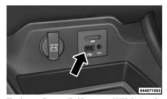
This feature allows an iPod® or external USB device to be plugged into the USB port.
