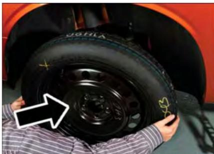
8. Install the lug nuts with the cone shaped end of the lug nut toward the wheel. Lightly tighten the lug nuts.
