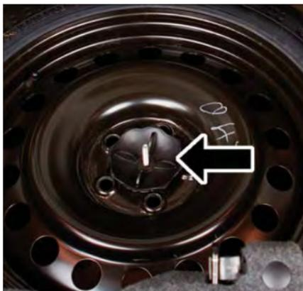
5. Remove the fastener securing the jack.
