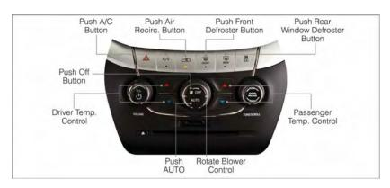
For your convenience the climate controls can be operated by using the soft-keys located on the touch screen or the climate control knobs below the Uconnect<sup>®</sup> display.
