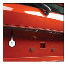
1 - Electronic Liftgate Lock/Unlock Pad
