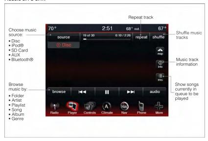
The iPod®/USB, CD, Audio Jack, SD Card or Bluetooth® source is accessed by touching the "Player" soft-key to enter the Player main screen, then touch the "Source" soft-key and choose between Disc, Aux, iPod®, Bluetooth® or SD Card.
