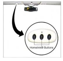
then press and hold the two outside HomeLink $^{\tiny (I)}$  buttons (I and III) for up to 20 seconds or until the red indicator flashes.
