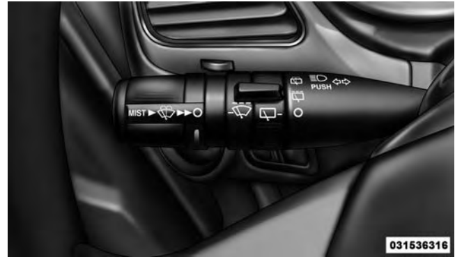
Windshield Wiper/Washer Lever
