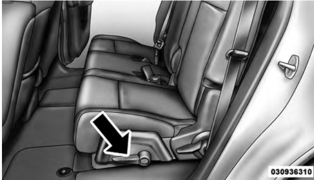
Seat Track Release Lever
