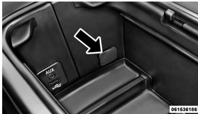
Shift Lever Override Access Cover
