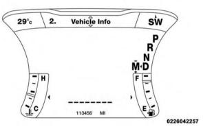
Driver Information Display (DID) Display This system conveniently allows the driver to select a variety of useful information by pushing the arrow
