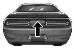
**NOTE:** If you inadvertently leave your vehicle's Passive Entry RKE transmitter in the trunk and try to close the deck lid, the deck lid will automatically unlatch, unless another one of the vehicle's Passive Entry RKE transmitters is outside the vehicle and within 5 ft (1.5 m) of the deck lid.
