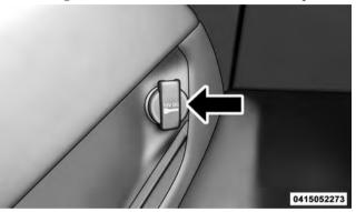
Power Outlet — Integrated Center Stack Front
