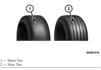
These indicators are molded into the bottom of the tread grooves. They will appear as bands when the tread depth becomes a 1/16 of an inch (2 mm). When the tread is worn to the tread wear indicators, the tire should be replaced. Refer to "Replacement Tires" in this section for further information.
