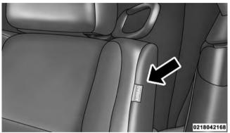
Front Supplemental Seat-Mounted Side Air Bag Label The SABs may help to reduce the risk of occupant injury during certain side impact and certain rollover events, in addition to the injury reduction potential provided by the seat belts and body structure.
