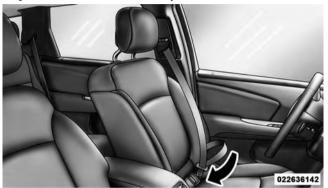
**Inserting Latch Plate Into Buckle**
