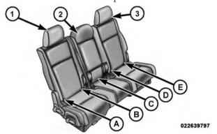
Options for installing two child seats using the LATCH anchorages in this vehicle:
