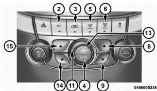
Automatic Temperature Controls — Buttons On The Faceplate
