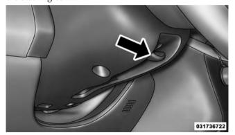
Tilt/Telescoping Steering Control Handle
