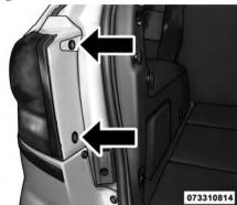
**Inboard Tail Lamp Housing Fasteners**
