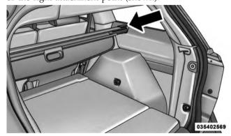
Installing Retractable Cargo Area Cover
