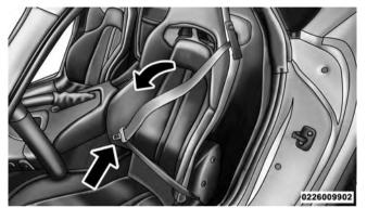
**Inserting Latch Plate Into Buckle**
