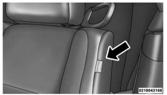
Front Supplemental Seat-Mounted Side Air Bag Label The SABs may help to reduce the risk of occupant injury during certain side impacts and/or vehicle rollover events, in addition to the injury reduction potential provided by the seat belts and body structure.
