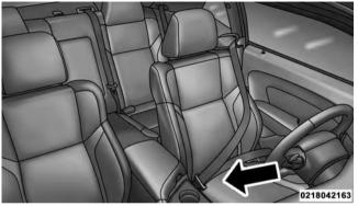
**Inserting Latch Plate Into Buckle**
