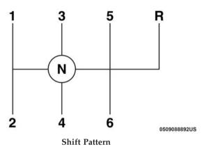
The six-speed manual transmission has a spring that centers the gear selector near third and fourth gear. This spring helps you know which gear you are in when you are shifting. Be careful when shifting from first to second or downshifting from sixth to fifth.
