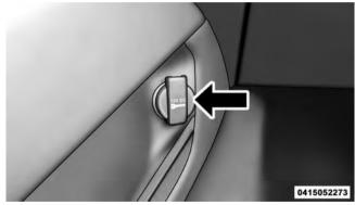
Power Outlet — Integrated Center Stack Front
