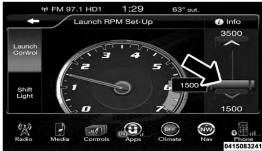
**Launch RPM Set-Up — Charger Automatic Transmission**
