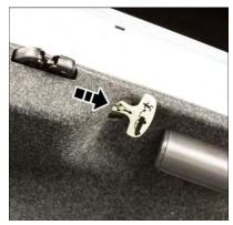
**Trunk Internal Emergency Release Lever**
