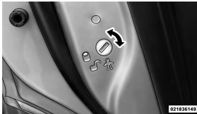
Child-Protection Door Lock Function
