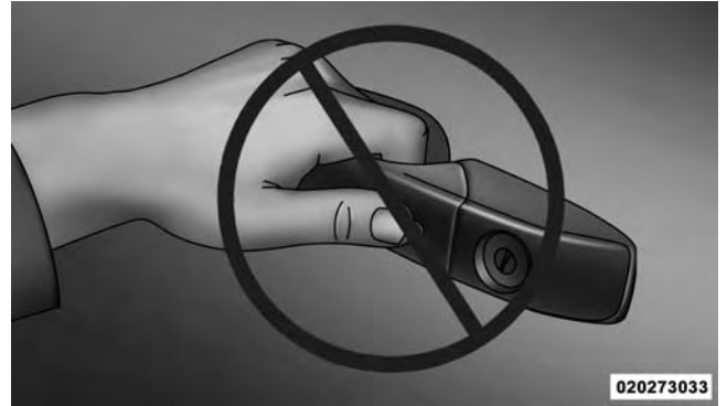
Do NOT Grab The Handle When Locking
