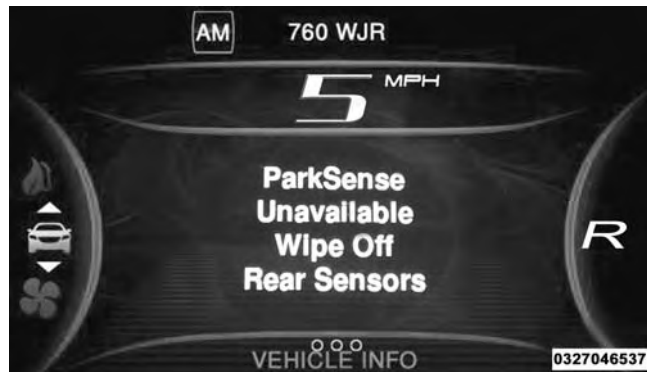
ParkSense Unavailable Wipe Off Rear Sensors
