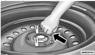
**Releasing Protective Plate Preparations For Jacking**
