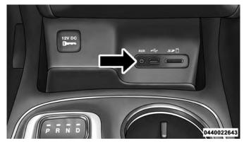
Integrated Center Console USB/AUX SD Card Media HUB Once the audio device is connected and synchronized to the vehicles iPod/USB/MP3 control system (iPod or external USB device may take a few minutes to connect), the audio device starts charging and is ready for use.
