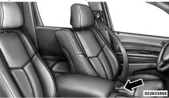
**Inserting Latch Plate Into Buckle**
