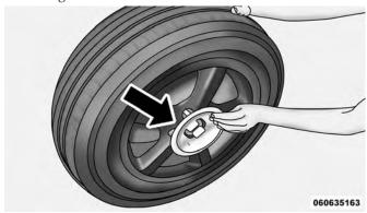
Installing Protective Plate On Damaged Wheel **NOTE:** The plastic plate will prevent the road wheel from being scratched when sliding it under the vehicle.
