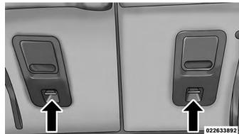
Top Tether Strap Anchorage (Located On Seatback)
