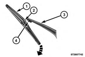
Removing The Wiper Blade
