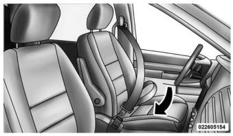
Inserting Latch Plate Into Buckle
