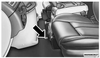
Winch Cover Assembly Plug (If Equipped)
