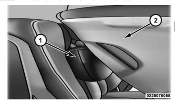
Car Seat With Head Restraint Folded
