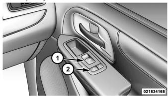
Front Passenger Power Window And Door Switches
