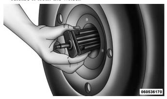
Removing Wheel Spacer
