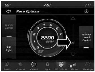
Launch RPM Set-Up
