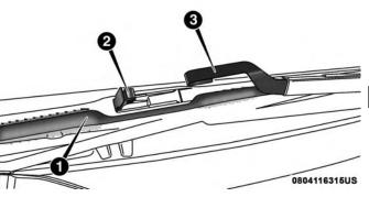
**Removing Wiper From Wiper Arm**
