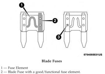
3 — Blade fuse with a NOT functional / BAD fuse element (blown fuse).
