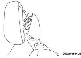
Active Head Restraint (AHR) Deployed
