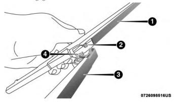
Wiper Blade Removed From Wiper Arm
