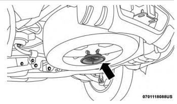
Road Wheel Installed In Spare Location
