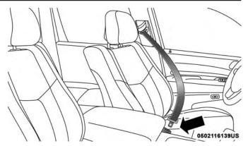
Inserting Latch Plate Into Buckle
