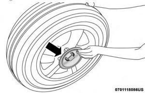
Installing Protective Plate On Damaged Wheel **NOTE:** The plastic plate will prevent the road wheel from being scratched when sliding it under the vehicle.
