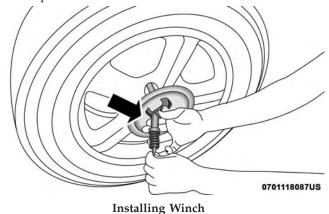
12. Slide the road wheel on the ground using the protective plate until it is directly under the winch and between the rear bumper and exhaust system heat shields. Raise the tire by turning the lug wrench on the winch extension clockwise until it clicks/ratchets three times to make sure the cable is tight.
