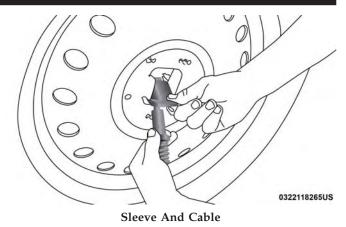
7. Pinch the three short and two long tubes to remove the protective plate from the steel spare wheel.
