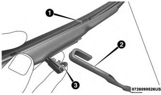
Wiper Blade Removed From Wiper Arm
