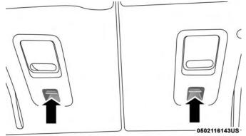
Top Tether Strap Anchorage (Located On Seatback)
