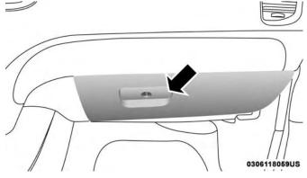
**Glove Compartment** To open the glove compartment, pull the release handle.
