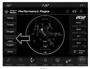
**G-Force** When selected, this screen displays all four G-Force values, as well as steering angle. When G-Force is selected, the following features will be available:
