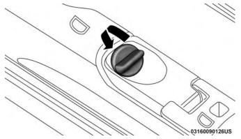
**Thumb Screw NOTE:** The thumb screws cannot be fully removed.
