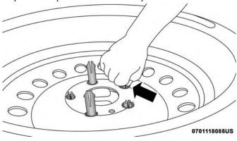
Releasing Protective Plate Preparations For Jacking
