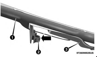
Wiper Blade With Release Tab In Unlocked Position
