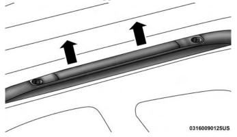
3. Starting with one crossbar, bend down the pivot supports at each end.
