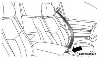
Inserting Latch Plate Into Buckle
