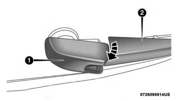
Wiper Pivot Cap In Unlocked Position
