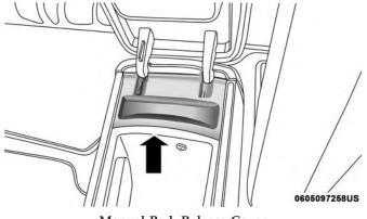
Manual Park Release Cover 3. Press and maintain firm pressure on the brake pedal.
