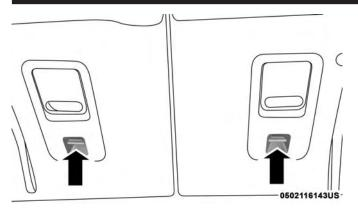
Top Tether Strap Anchorage (Located On Seatback)
