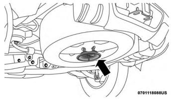
Road Wheel Installed In Spare Location
