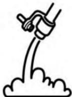
Push in the Mode Select Knob and turn to this position to inject the Tire Service Kit Sealant and to inflate the tire.
