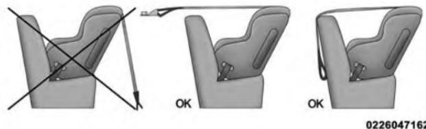
1. Look behind the seating position where you plan to install the child restraint to find the tether anchorage. You may need to move the seat forward to provide better access to the tether anchorage. If there is no top tether anchorage for that seating position, move the child restraint to another position in the vehicle if one is available.
