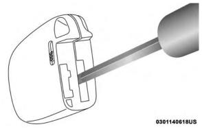
Separating Case With A Flat Blade Screwdriver
