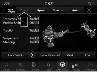
Your SRT vehicle is equipped with a Drive Modes feature which allows for coordinating the operation of various vehicle systems depending upon the type of driving behavior desired. The Drive Modes feature is controlled through the Uconnect system and may be accessed by performing any of the following:
