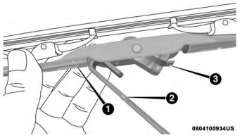
Wiper Blade Removed From Wiper Arm
