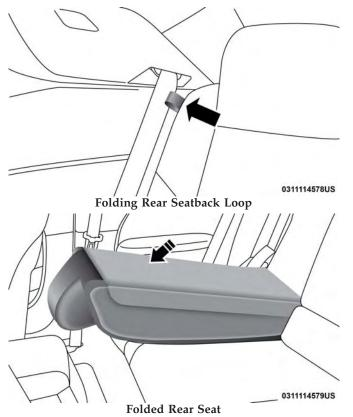
When the seatback is folded to the upright position, make sure it is latched by strongly pulling on the top of the seatback above the seat strap.
