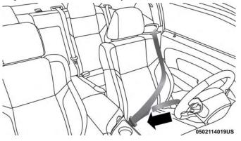
Inserting Latch Plate Into Buckle
