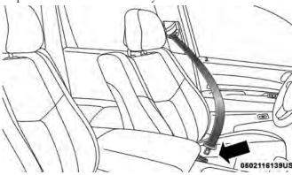
Inserting Latch Plate Into Buckle
