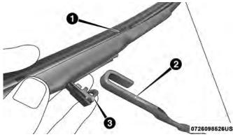
Wiper Blade Removed From Wiper Arm
