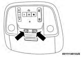
Front Map/Reading Light Switches Ambient Light — If Equipped
