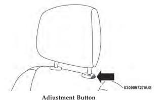
For comfort the Active Head Restraints can be tilted forward and rearward. To tilt the head restraint closer to the back of your head, pull forward on the bottom of the head restraint. Push rearward on the bottom of the head restraint to move the head restraint away from your head. 3
