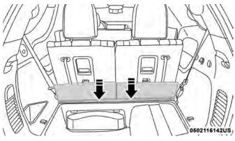
Pulling Down The Carpet Floor Panel To Access Top Tether Strap Anchorage (3rd Row Bench)
