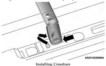
6. Deploy and tighten the second crossbar to complete the deployment of the crossbars.
