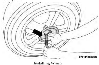
12. Slide the road wheel on the ground using the protective plate until it is directly under the winch and between the rear bumper and exhaust system heat shields. Raise the tire by turning the lug wrench on the winch extension clockwise until it clicks/ratchets three times to make sure the cable is tight.
