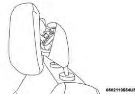
Active Head Restraint (AHR) Deployed
