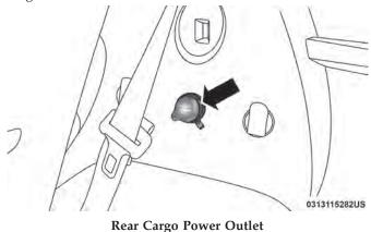
**NOTE:** The rear cargo power outlet can be changed to "battery" powered all the time by switching the power outlet right rear quarter panel fuse in the fuse panel from fuse location F90 to F91.
