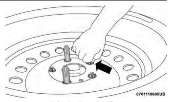
Releasing Protective Plate **Preparations For Jacking**
