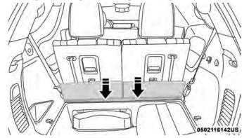
Pulling Down The Carpet Floor Panel To Access Top Tether Strap (3rd Row Bench)
