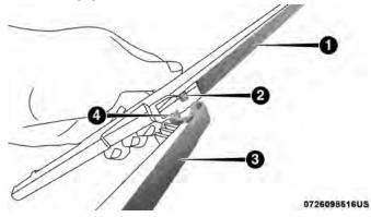
Wiper Blade Removed From Wiper Arm
