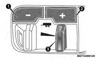
**Integrated Trailer Brake Module (ITBM)**
