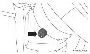
Power Tilt/Telescoping Steering Column
