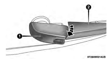
Wiper Pivot Cap In Unlocked Position
