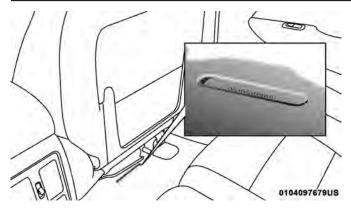
Right Front Body VIN Location **NOTE:** It is illegal to remove or alter the VIN.
