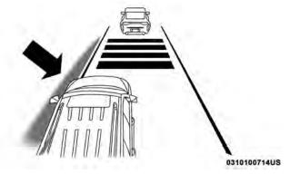
Lane Approached (Flashing Yellow Thick Line, Solid Yellow Thin Line/Flashing Yellow Telltale (3)
