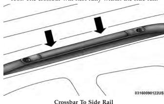
5. Once the driver's side crossbar is in place, tighten the thumb screws completely.
