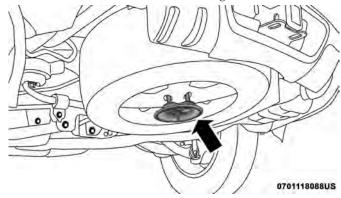
Road Wheel Installed In Spare Location
