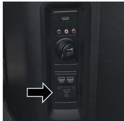
Power Inverter Outlet
