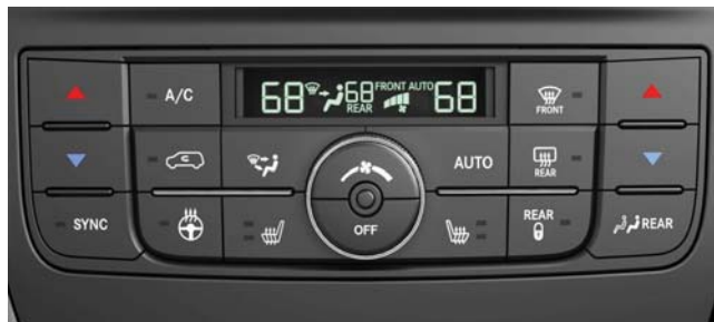
Automatic Temperature Controls
