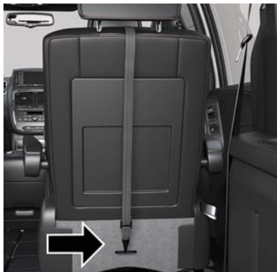
Tether Strap Anchorages (Second Row Captains Chair Anchorage Shown)
