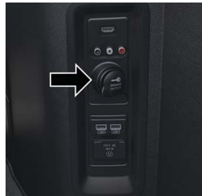
Rear Panel Power Outlet
