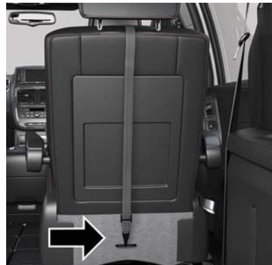
Rear Seat Tether Strap Mounting (Second Row Bench Anchorage Shown)
