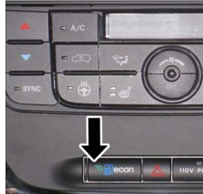
ECON Switch Location
