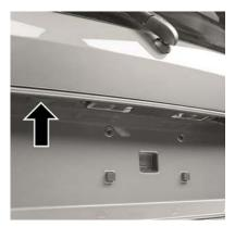
**Electronic Liftgate Lock/Unlock Pad**
