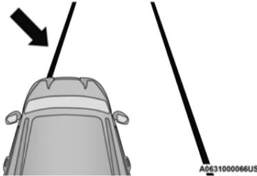
**Lane Approached (Flashing Yellow Line With Flashing Yellow Telltale)
