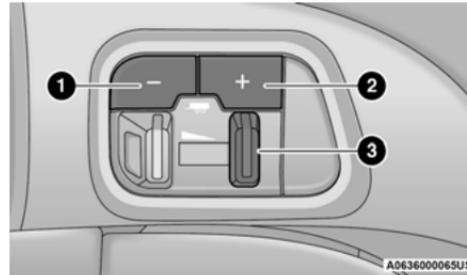
**Integrated Trailer Brake Module (ITBM)**
