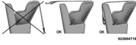
1. Look behind the seating position where you plan to install the child restraint to find the tether anchorage. You may need to move the seat forward to provide better access to the tether anchorage. If there is no top tether anchorage for that seating position, move the child restraint to another position in the vehicle if one is available.
