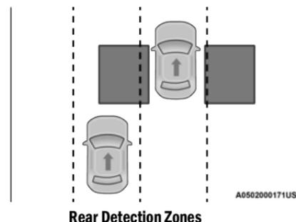
When the vehicle is started, the BSM Warning Light will momentarily illuminate in both outside rearview mirrors to let the driver know that the system is operational. The BSM system sensors operate when the vehicle is in any forward gear or REVERSE (R).
