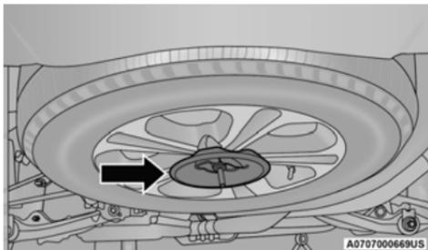
**Road Wheel Installed In Spare Location**
