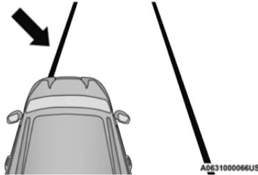
**Lane Approached (Flashing Yellow Line With Flashing Yellow Telltale)
