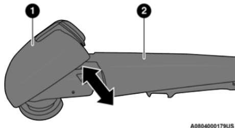
**Wiper Pivot Cap In Unlocked Position**
