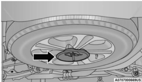
**Road Wheel Installed In Spare Location**
