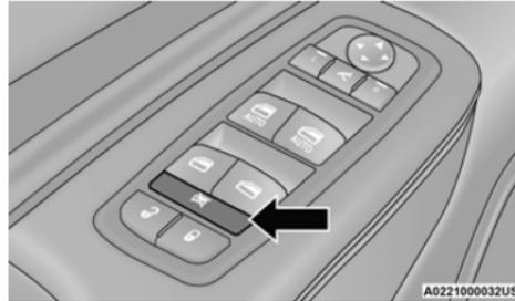
**Power Window Lockout Switch****WIND BUFFETING**
