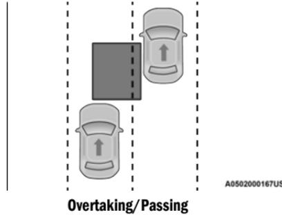
The BSM system is designed not to issue an alert on stationary objects such as guardrails, posts, walls, foliage, berms, etc. However, occasionally the system may alert on such objects. This is normal operation and your vehicle does not require service.
