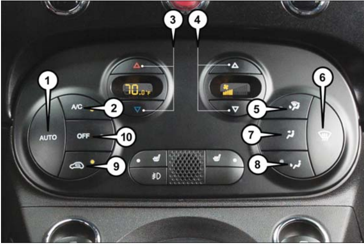
Automatic Temperature Controls
