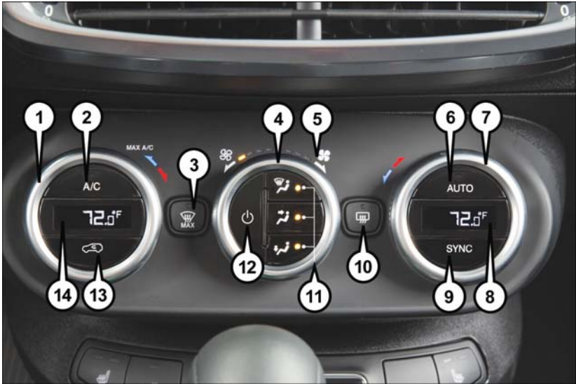
Automatic Temperature Controls (ATC)
