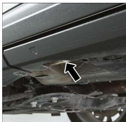
Front Jacking Location
