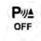
When the ParkSense switch is pushed to disable the system, the instrument cluster will display the “PARKSENSE OFF” message for
