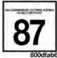
All available gasoline engines are designed to meet all emissions regulations and provide excellent fuel economy and performance when using high quality unleaded “regular” gasoline having a octane rating of 87 using the (R+M)/2 method. The use of premium gasoline is not recommended, as it will not provide any benefit over regular gasoline in these engines.
