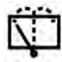
To use the washer, push the lever forward and hold while spray is desired. If the lever is pushed while in the intermittent setting, the wiper will turn on and operate for several wipe cycles after the end of the lever is released, and then resume the intermittent interval previously selected.
