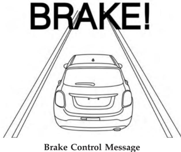
When the system determines a collision with the vehicle in front of you is no longer probable, the warning message will be deactivated.
