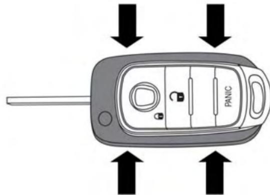
Integrated Vehicle Key Battery Removal
