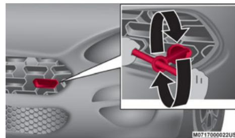
**Installing Front Towing Eye**
