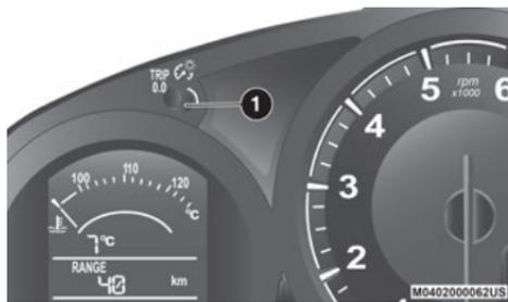
**Odometer/Trip Reset Button**
