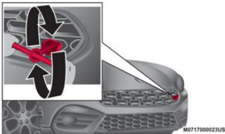
**Abarth Installing Front Towing Eye**
