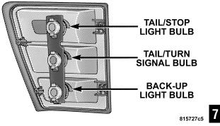
4. Pull the bulb to remove it from the socket. 81572594
