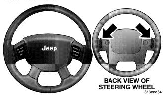
The right hand control is a rocker type switch with a push-button in the center and controls the volume and mode of the sound system. Pressing the top of the rocker switch will increase the volume and pressing the bottom of the rocker switch will decrease the volume.
