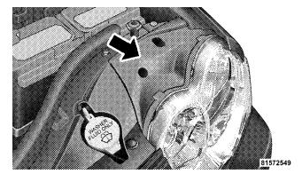
3. Turn the turn signal bulb 1/4 turn counter clockwise to remove from housing.
