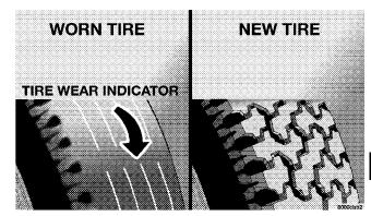
These indicators are molded into the bottom of the tread grooves and will appear as bands when the tread depth becomes 1/16 inch (2 mm). When the indicators appear in 2 or more adjacent grooves, the tire should be replaced.
