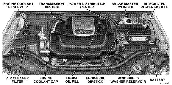
**ENGINE COMPARTMENT – 3.0L DIESEL**
