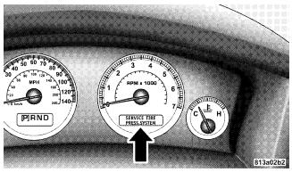
The Electronic Vehicle Information Center (EVIC) features a driver-interactive display. It is located on the bottom of the tachometer in the instrument cluster. The EVIC consists of the following:
