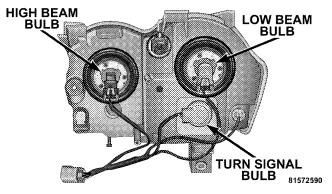
3. Disconnect the electrical connector and replace the bulb.
