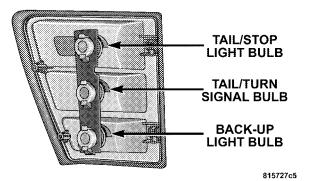
4. Pull the bulb to remove it from the socket.
