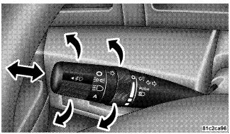
Headlight Switch Automatic Headlight System — If Equipped Turn the end of the multi-function control lever to the third detent to activate the automatic headlight system. This system performs two functions. With the engine running and the multi-function control lever in the A (Auto) position, the headlights will turn on and off based on the surrounding light levels.
