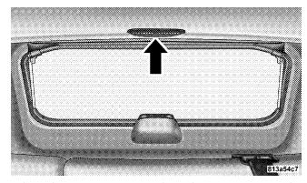
When the ignition is turned to the ON position, the warning display will turn ON all of its LEDs for about one second. Each side of the warning display has six yellow and two red LEDs. The vehicle is close to the obstacle when the red LED is ON.
