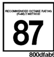
Your engine is designed to meet all emissions regulations and provide excellent fuel economy and performance when using high quality unleaded “regular” gasoline having an octane rating of 87. The use of premium gasoline is not recommended, as it will not provide any benefit over regular gasoline in these engines.
