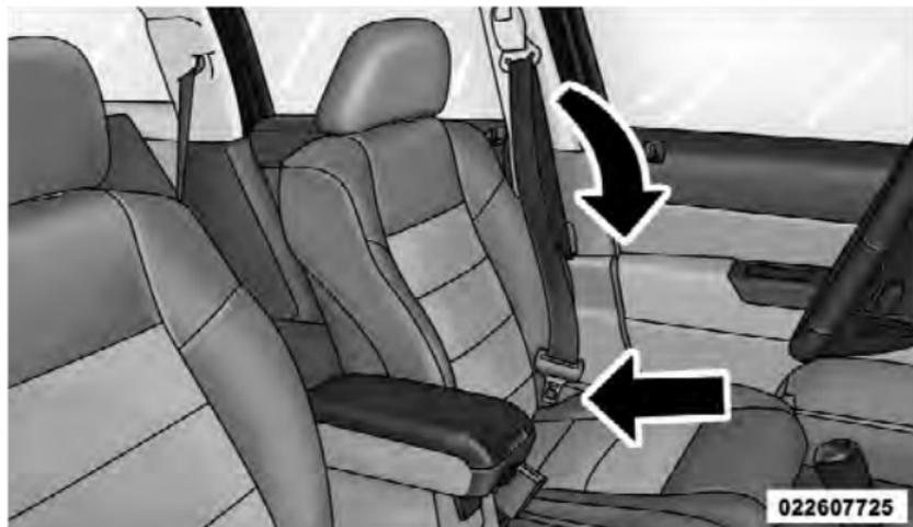
Inserting Latch Plate Into Buckle
