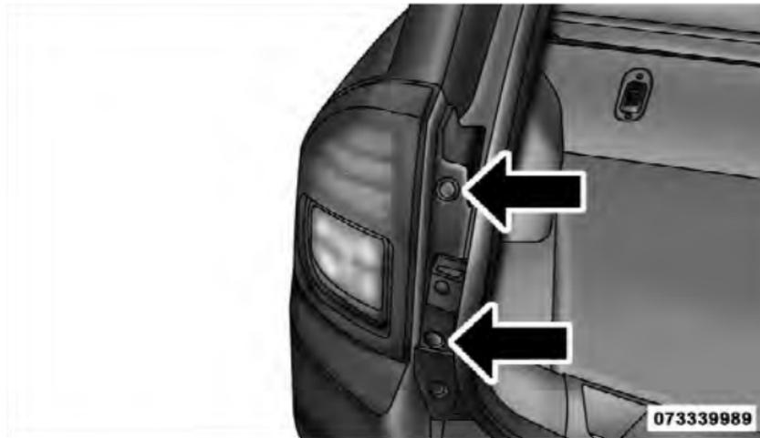
2. Grasp the taillamp and pull firmly to disengage the lamp from the aperture panel.
