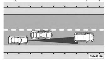
When driving on a curve with ACC engaged, the system may decrease the vehicle speed and acceleration for convenience reasons, with no target vehicle detected. Once the vehicle is out of the curve the system will resume your original Set Speed. This is a part of normal ACC system functionality.
