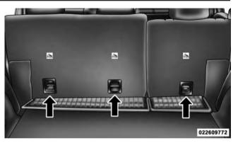
Top Tether Strap Anchorage (Located on Seatback)
