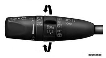
Rotate the center portion of the lever upward to the first detent for intermittent operation and to the second detent for continuous rear wiper operation.
