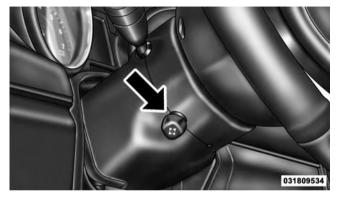
Power Tilt/Telescoping Steering Column
