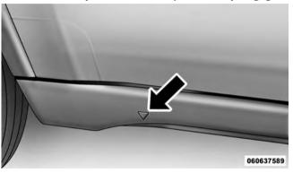
Lift Point Symbol On Sill Molding
