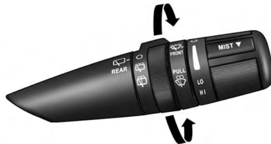
Rear Wiper/Washer Control Lever
