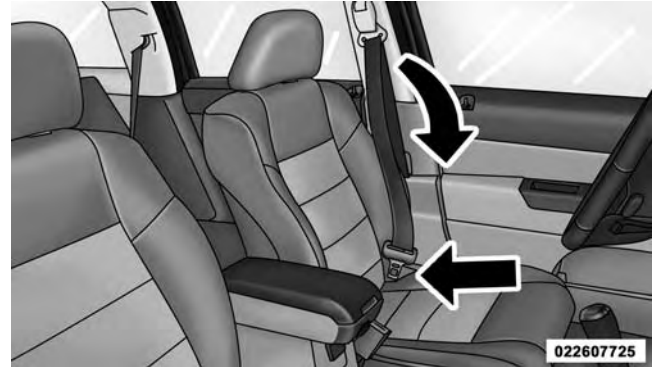
Inserting Latch Plate Into Buckle
