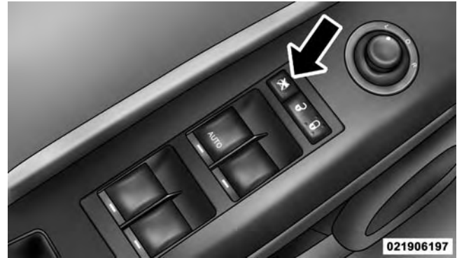
Window Lockout Switch
