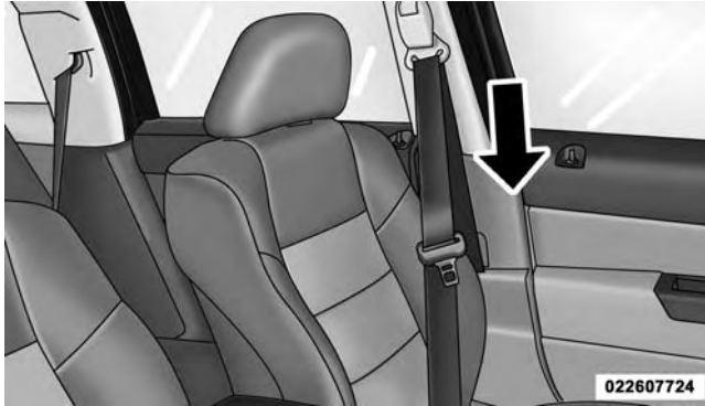
Pulling Out The Latch Plate
