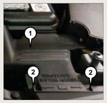
Air Intake Duct/Finger Screws
