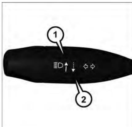
Turn Signal/High Beam Lever
