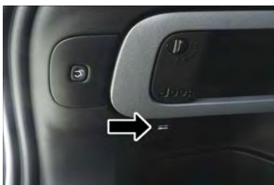
Rear Cargo Power Outlet
