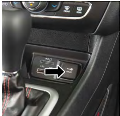
Front Power Outlet
