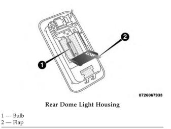
3. Insert the new bulb, locking it between the contacts.
