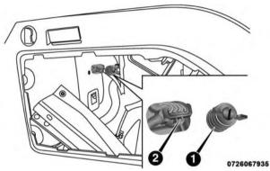
**Rear Lamp Fastener and Electrical Connector**
