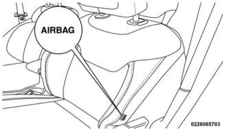
**Front Supplemental Seat-Mounted Side Air Bag** The SABs may help to reduce the risk of occupant injury during certain side impacts and/or vehicle rollover events, in addition to the injury reduction potential provided by the seat belts and body structure.
