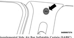
Supplemental Side Air Bag Inflatable Curtain (SABIC) Label Location SABICs may help reduce the risk of head or other injuries to front and rear seat outboard occupants in certain side impacts and/or vehicle rollover events, in addition to the injury reduction potential provided by the seat belts and body structure.
