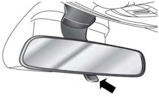
**Mirror Adjustment NOTE:** The mirror will automatically release in the event of heavy contact with a passenger.
