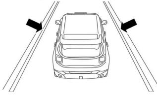
• When the LaneSense system senses the lane has been approached and is in a lane departure situation, the left thick lane line flashes yellow (on/off) and the left thin line remains solid yellow. The LaneSense indicator changes from solid yellow to flashing yellow. At this time torque is applied to the steering wheel in the opposite direction of the lane boundary.
