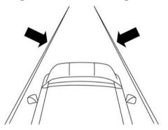
Lane Sensed (Solid White Thick Line, Solid White Thin Line/Solid Yellow Indicator) • When the LaneSense system senses the lane has been approached and is in a lane departure situation, the left thick lane line flashes from white to gray, the left thin line remains solid white and the LaneSense indicator changes from solid yellow to flashing yellow. At this time, torque is applied to the steering wheel in the opposite direction of the lane boundary.
