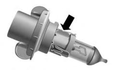
5. Install the headlamp bulb and socket; turn it clockwise making sure it is properly locked.
