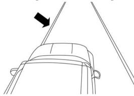
Lane Approached (Flashing White To Gray Thick Line, Solid White Thin Line/Flashing Yellow Indicator) NOTE: The LaneSense system operates with the similar behavior for a right lane departure.
