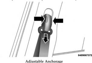
As a guide, if you are shorter than average, you will prefer the shoulder belt anchorage in a lower position, and if you are taller than average, you will prefer the shoulder belt anchorage in a higher position. After you release the anchorage button, try to move it up or down to make sure that it is locked in position.
