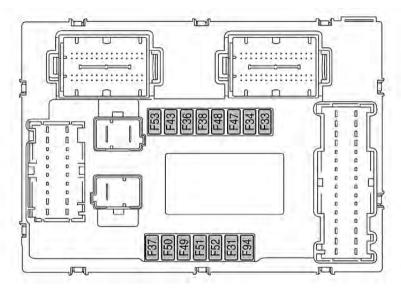
**Body Controller Fuse Cavities**
