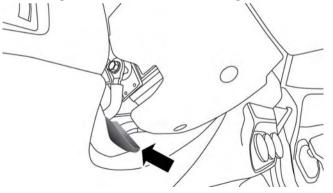
To unlock the steering column, push the tilt/telescoping lever downward (toward the floor). To tilt the steering column, move the steering wheel upward or downward as desired. To lengthen or shorten the steering column, pull the steering wheel outward or push it inward as desired.
