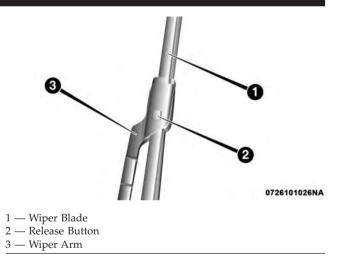
4. Install the wiper blade and firmly push the wiper blade until it snaps into place.
