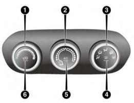
Manual Temperature Controls (MTC) The Manual Climate Controls consist of a series of rotary dials with inner push buttons.
