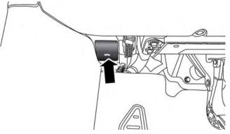
Move to the outside of the vehicle and push the safety latch release lever toward the passenger side of the vehicle. The hood release lever is located behind the center front edge of the hood.
