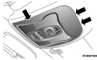
2. Release the retainer clips and bulb housing as shown.
