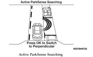
When an available parking space has been found, and the vehicle is not in position, you will be instructed to move forward to position the vehicle for a parallel parking sequence.
