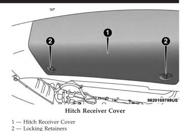
2. Pull the bottom of the cover outward (towards you), pull downwards to disengage the tabs located at the top of the hitch receiver cover.
