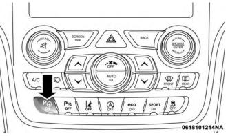
**ParkSense Active Park Assist Switch Location** To enable the ParkSense Active Park Assist system, push the ParkSense Active Park Assist switch once (LED turns on). To disable the ParkSense Active Park Assist system, push the ParkSense Active Park Assist switch again (LED turns off).
