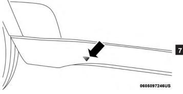
Lift Point Symbol On Sill Molding
