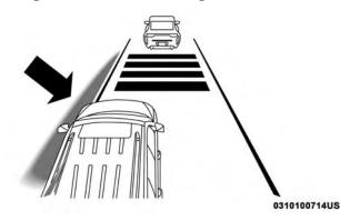
Lane Approached (Flashing Yellow Thick Line, Solid Yellow Thin Line/Flashing Yellow Telltale) NOTE: The LaneSense system operates with the similar behavior for a right lane departure.
