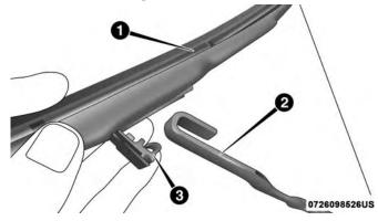
Wiper Blade Removed From Wiper Arm
