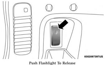
To operate the flashlight, push the switch once for high, twice for low, and a third time to return to off.
