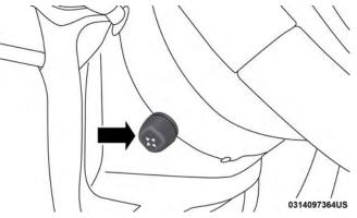
Power Tilt/Telescoping Steering Column
