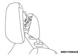
Active Head Restraint (AHR) Triggered
