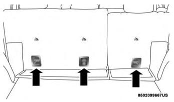
Top Tether Strap Anchorage (Located On Seatback)
