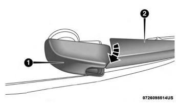
Wiper Pivot Cap In Unlocked Position
