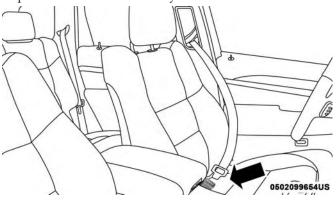
Inserting Latch Plate Into Buckle
