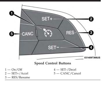
**NOTE:** In order to ensure proper operation, the Speed Control System has been designed to shut down if multiple Speed Control functions are operated at the same time. If this occurs, the Speed Control System can be reactivated by pushing the Speed Control on/off button and resetting the desired vehicle set speed.
