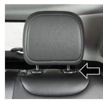
Outboard Head Restraint Adjustment Button
