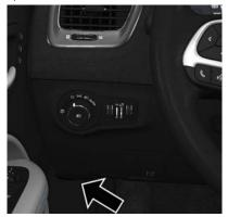
Hood Release Location (Underneath Instrument Panel)
