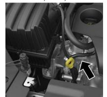
Suitable Engine Ground (Example Engine Shown)
