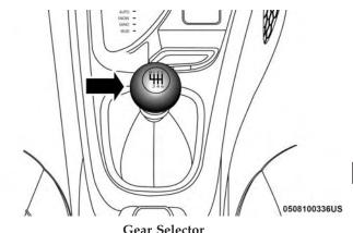
To shift the gears, fully press the clutch pedal and place the gear selector into the desired gear position (the diagram for the engagement of the gears is displayed on the handle of the selector).
