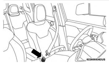
Inserting Latch Plate Into Buckle
