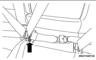
**Inserting Latch Plate Into Buckle**
