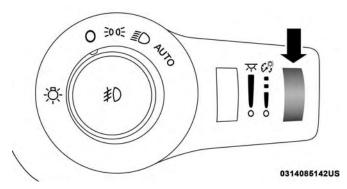
Instrument Panel Dimmer Ambient Light Control — If Equipped
