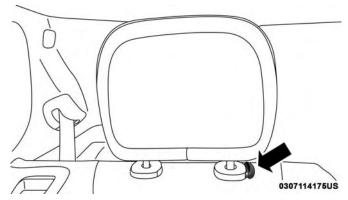
Outboard Head Restraint Adjustment Button
