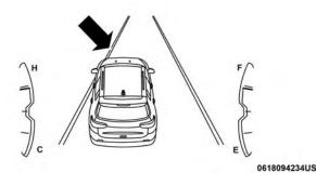
Lane Approached (Flashing White To Gray Thick Line, Solid White Thin Line/Flashing Yellow Telltale (\$\mathcal{G}\)) NOTE: The LaneSense system operates with the similar behavior for a right lane departure.
