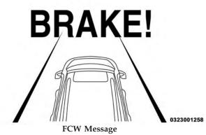
When the system determines a collision with the vehicle in front of you is no longer probable, the warning message will be deactivated.
