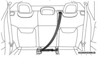
**Inserting Latch Plate Into Buckle**
