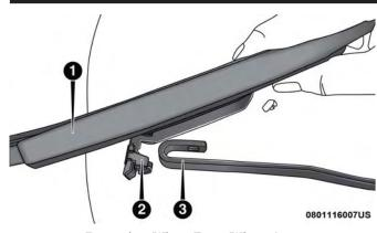
Removing Wiper From Wiper Arm
