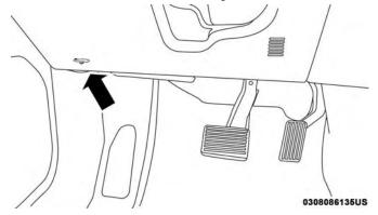
Hood Release Location (Underneath Instrument Panel)
