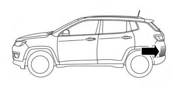
Radar Sensor Location (Driver Side Shown)
