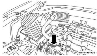
Suitable Engine Ground (Example Engine Shown)
