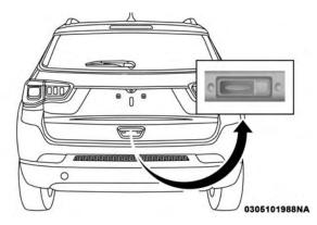
Electronic Liftgate Release/Liftgate Passive Entry Location
