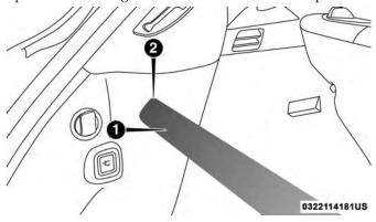
Raised Load Floor — (Power Liftgate)
