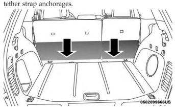
Pulling Down The Carpet Floor Panel To Access Top Tether Strap Anchorage
