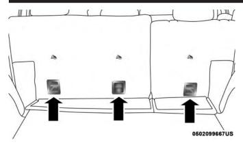
Top Tether Strap Anchorage (Located On Seatback)
