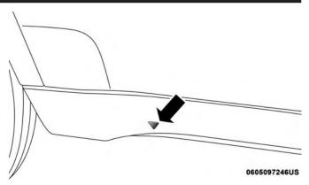
Lift Point Symbol On Sill Molding
