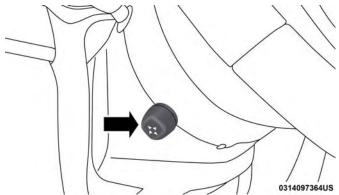
Power Tilt/Telescoping Steering Column
