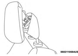
Active Head Restraint (AHR) Deployed
