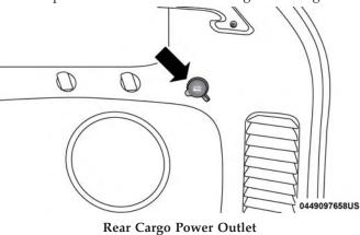
NOTE: The rear power outlet can be switched from switched "ignition" only to constant "battery" powered all the time. See your local authorized dealer for details.
