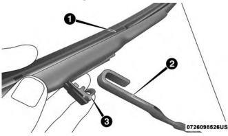
Wiper Blade Removed From Wiper Arm
