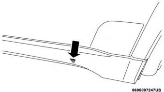
Lift Point Symbol On Sill Molding
