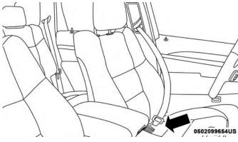
Inserting Latch Plate Into Buckle
