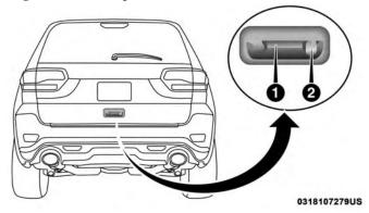
Electronic Liftgate Release/Liftgate Passive Entry Location
