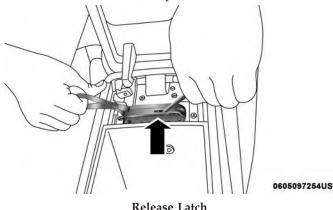
5. While the metal latch is in the open position, pull upward on the tether strap until the lever clicks and latches in the released position. The transmission is now out of PARK and the vehicle can be moved.
