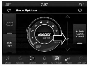
Launch RPM Set-Up
