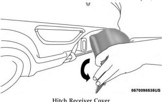
3. Lower back down to disengage the tabs located at the top of the hitch receiver cover and then pull outwards to remove.
