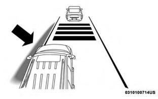
Lane Approached (Flashing Yellow Thick Line, Solid Yellow Thin Line/Flashing Yellow Telltale (\$\mathcal{Q}\))
