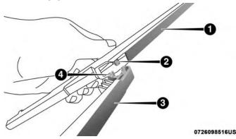
Wiper Blade Removed From Wiper Arm
